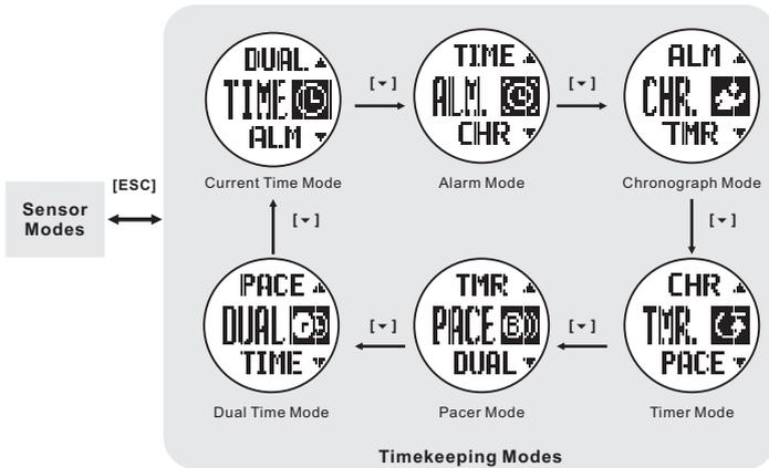
\* Press the [->] button to move the selection in the reverse direction.
