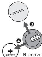
Remove the battery door and take away the old battery.
