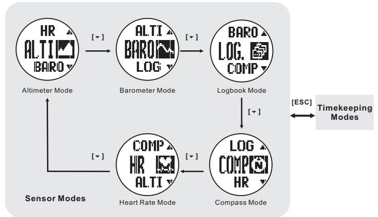
\* Press the [->] button to move the selection in the reverse direction.
